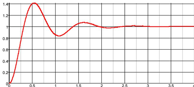
The simulation suggests that a fast 2 inch read will actually move to 2.8 inches before finally settling to 2 inches. This amount of overshoot was observed in practice. The simulation also suggests that the needle will take more than 2 seconds to settle (the horizontal scale of the graph is in seconds) which again was seen in practice.
